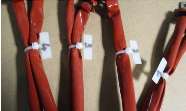
Cable connection according to the marks (from 1 to 4)
